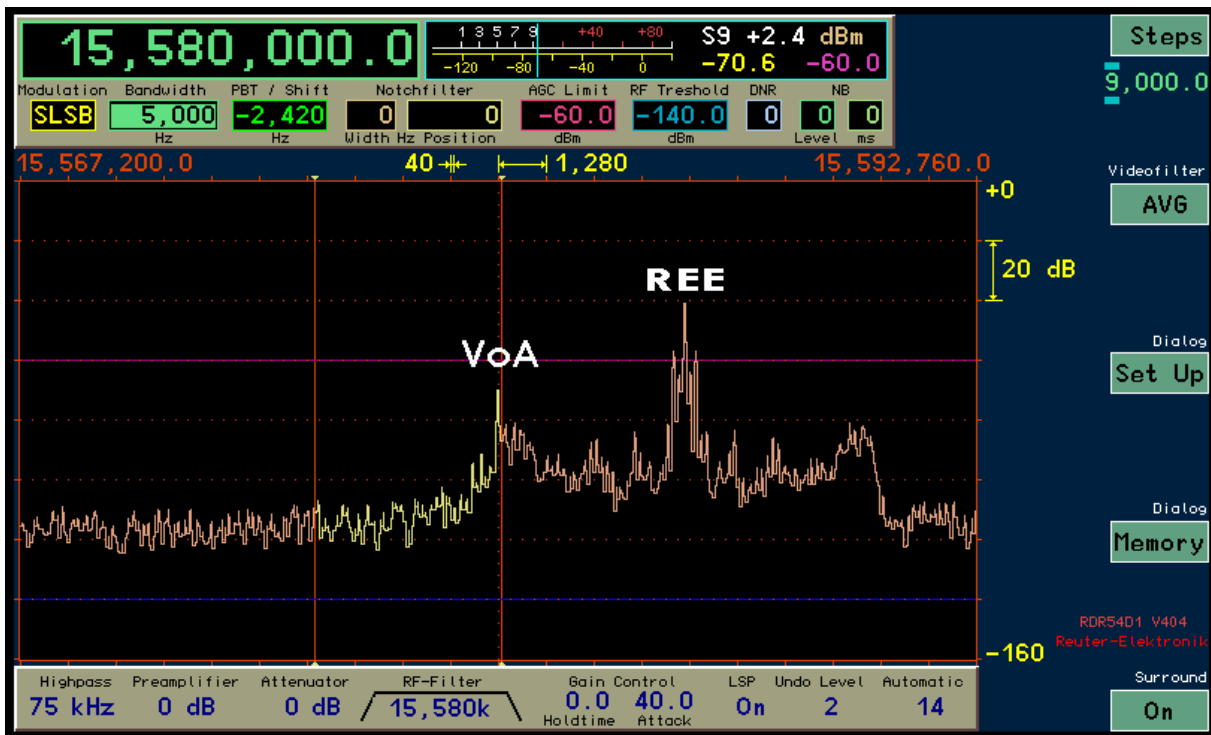
VoA reception using the Synchronous detector and LSB as an option. Audio and sideband bandwidth set to 5000 Hz.
