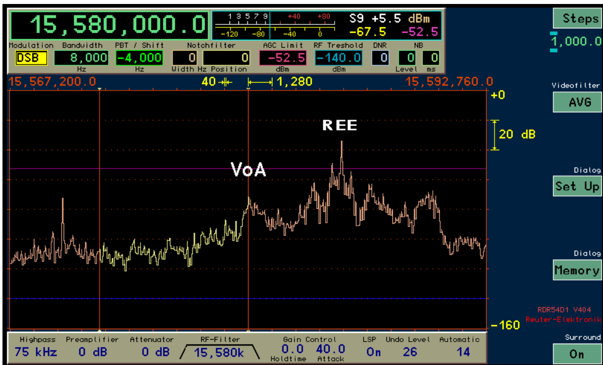
VoA reception using DSB and a Passband shift of 4000 Hz to cut out the REE signal completely. Note that the bandwidth needs to be adjusted afterwards also.
